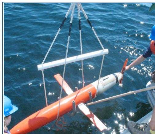
Figure 6. While the Spray requires no specialized launch and recovery equipment, customized equipment can be tailored to customer needs.
