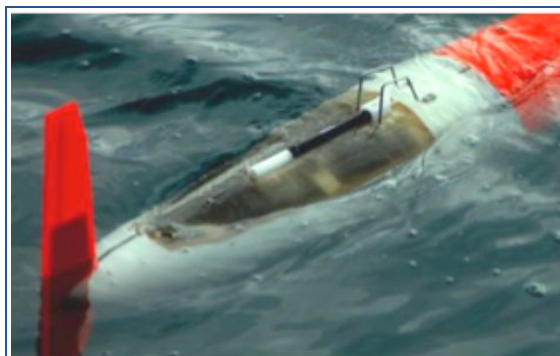
Figure 4. The Spray Glider's free-flooded sensor bay.
